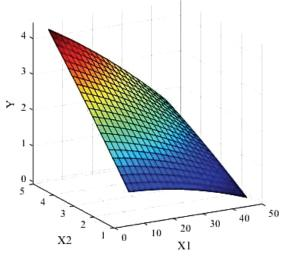
**Figure 1.** 3D surfaces for predicting the residual Fe<sup>3+</sup> concentration
