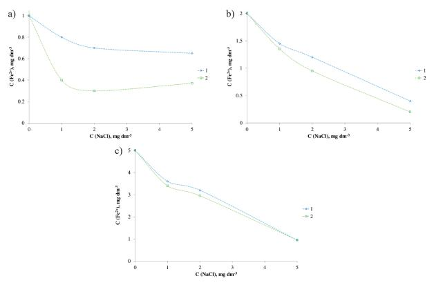
Figure 2. The effect of mineralization on the content of divalent ferrous iron (1 – comparison solution, 2 – model solution):  $a - C_{init} = 1 \text{ mg/dm}^3$ ,  $b - C_{init} = 2 \text{ mg/dm}^3$ ,  $c - C_{init} = 5 \text{ mg/dm}^3$
